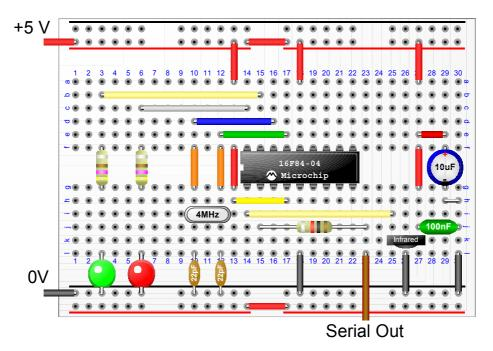
Fig 4. Possible solderless breadboard layout of above circuit..
