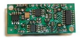
Connections to the SRF04 are via four of its five PCB pads shown below.
