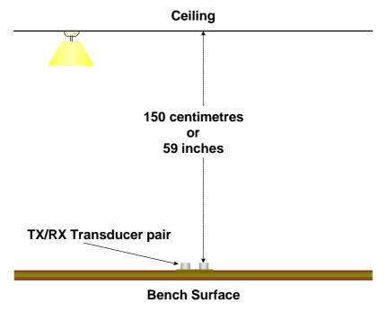
Dividing the raw distance of 8642 by 150 gives a value of 57.6, so without using floating point, our calculation to convert to centimetres is a simple division by 58: -
