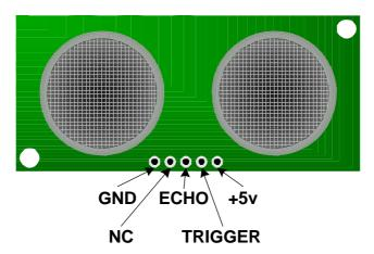
As far as I can tell, there is no polarity protection or voltage regulation on the PCB, so the SRF04 must be supplied with no more than 5 Volts, and the correct polarity must be observed otherwise damage 'will' occur.
