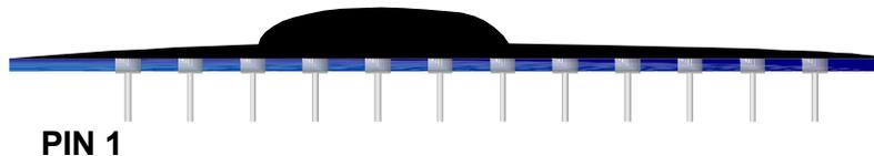
**Pins 1 and 2** are for connecting 2 optional LEDs, one **Red** and one **Green**. When the QuickBlue™ Link is in discovery mode, both LEDs will blink alternately, once a connection has been established, the **Green** LED will remain illuminated, while the **Red** LED blinks. Both pins have internal current limiting resistors, allowing direct connection of the LEDs.
