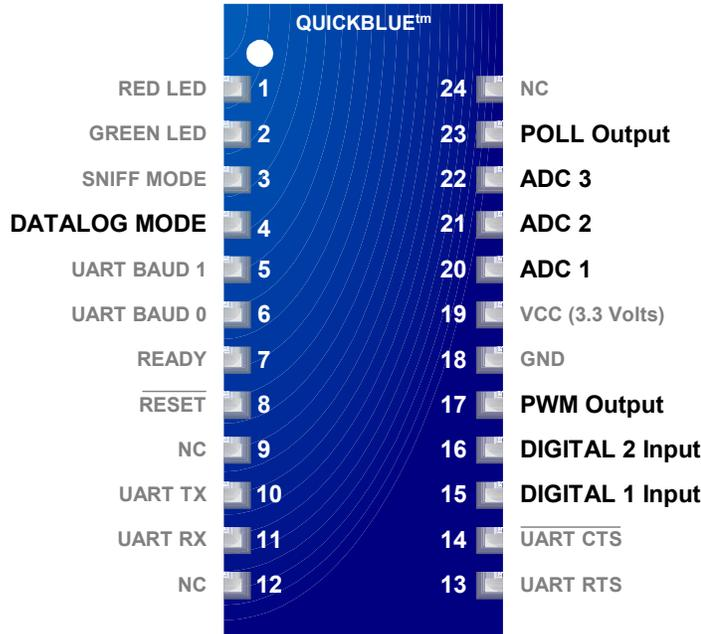
**POLL** is an output that strobes Low-High-Low for 1ms before scanning the ports and outputting the comma delimited string.
