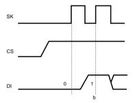
Fig. 9 Normal operation timing
