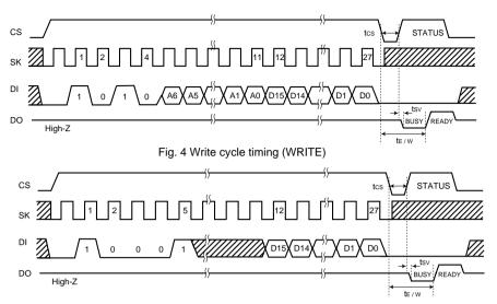
Fig. 5 Write all address cycle timing (WRAL)
